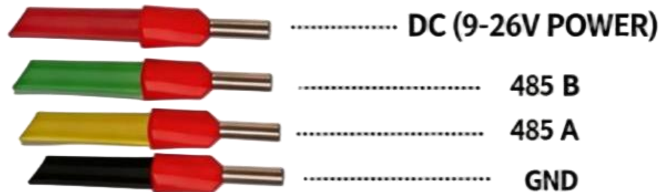
Fig. 4-1 RS485 Wiring Schematic
